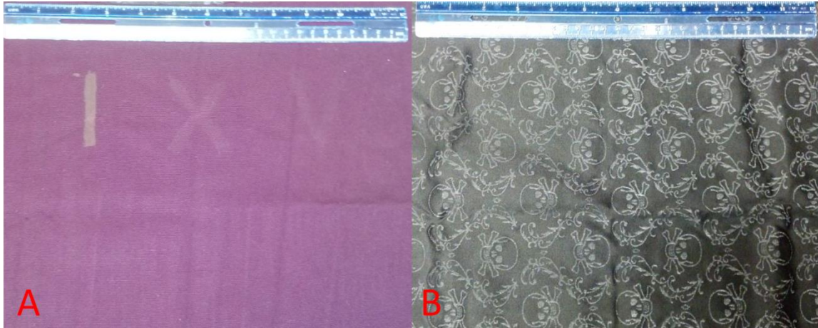
Figure 4.1 Image A shows the acrylic fabric with a 12-inch ruler. One can observe the 'I', the 'X', and the 'V', but the other two bloodstains are not visible. Image B shows the polyester fabric with the sewn-in skull prints. The bloodstains are not visible even with close examination. The skull pattern is the type that is ironed onto the fabric during production.
